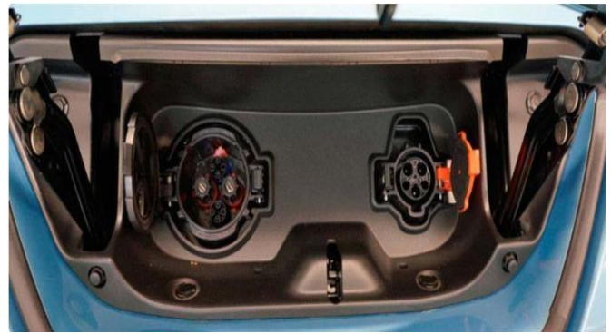
Figure 12. Nissan Leaf Mode 4 CHAdeMO (left) and Mod 3 socket(right) [25].
